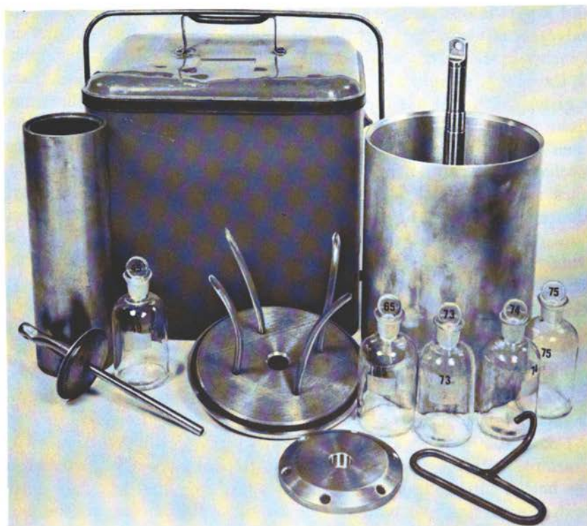
FIGURE 3.—Apparatus for sampling water that contains dissolved gases and constituents susceptible to aeration.
